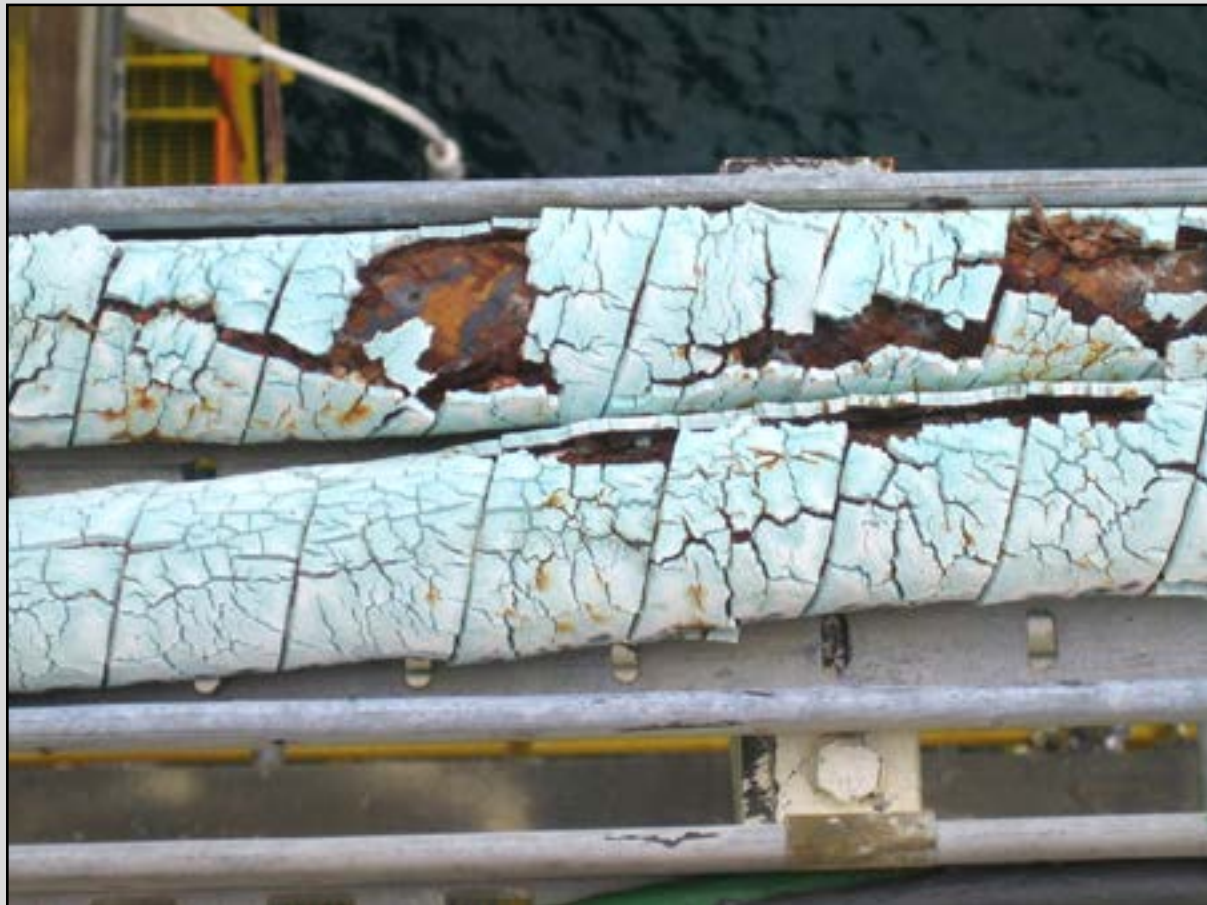
UV6 Cracked sheath, rusting armour
