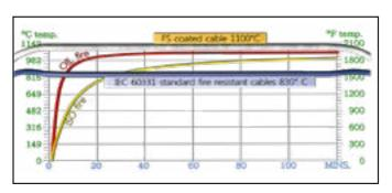
The yellow curve shows the temperature of an ISO fire - 830° Celsius, which is a normal cellulose fire.
