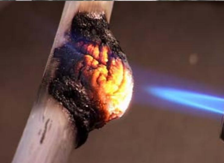
FS1 is an intumescent coating that will expand 100 times its thickness during a fire - thus protecting the cables from fire damage and making sure the cables function when needed the most.
