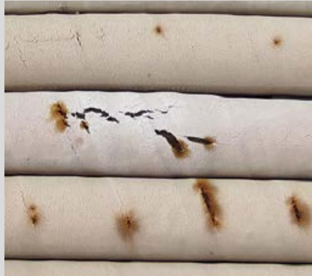
*FS Coating enhances the cables UV resistance, ozone resistance and increases the dielectric strength.*
