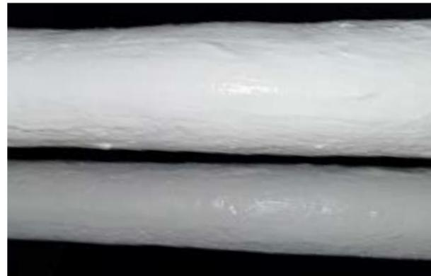
**HV Cables with fire damaged outer sheaths will usually be replaced**
