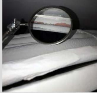
These examples are accepted FS Standard and Guaranteed that unprotected areas will achieve correct protection in the event of a fire, due to the fact that upon direct flame contact the chemical reaction starts and conceals areas with insulating foam that is released.
