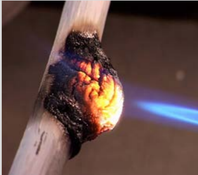
FS coatings restore and upgrade the cable's fire protection, reduces the toxicity release and delays short circuiting in a fire scenario.
