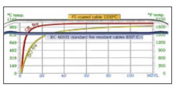
The yellow curve shows the temperature of an ISO fire -  $830^{\circ}$  Celsius, which is a normal cellulose fire. The red curve represents the temperature of an oil fire - up to  $1100^{\circ}$  Celsius - the temperature to which Fire Security has tested their coatings. This is the temperature you would be facing if you had such a fire.
