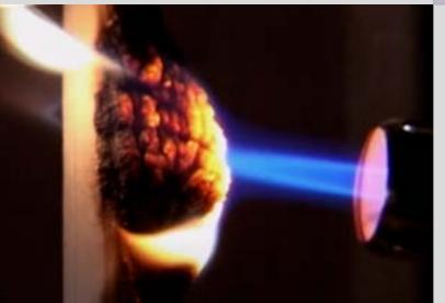
FS1 is an intumescent coating that will expand 100 times its thickness during a fire - thus protecting the cables from fire damage and making sure the cables function when needed the most.
