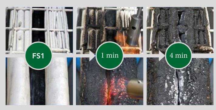
FS1 Intumescent coating product will expand up to 100-times its original thickness. As the coating expands, it becomes considerably more voluminous creating a lightweight char insulator that keeps high temperature away from cable cores and structural members, such as cable supports and cable trays.
